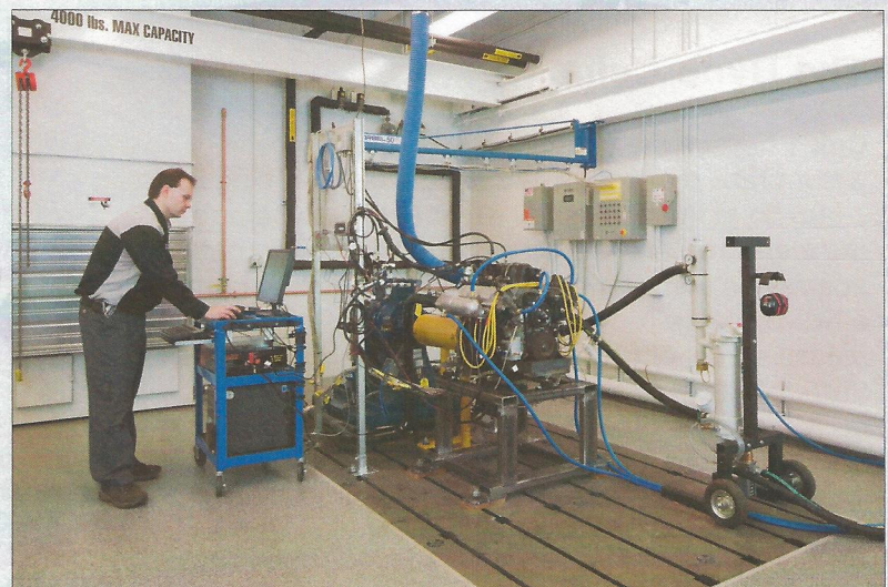
The GM 3800 Series II 3.8L V6 gasoline engine hooked up to the Midwest 1014 dynamometer allows in-depth testing and measuring of deposits, wear and oil durability.
